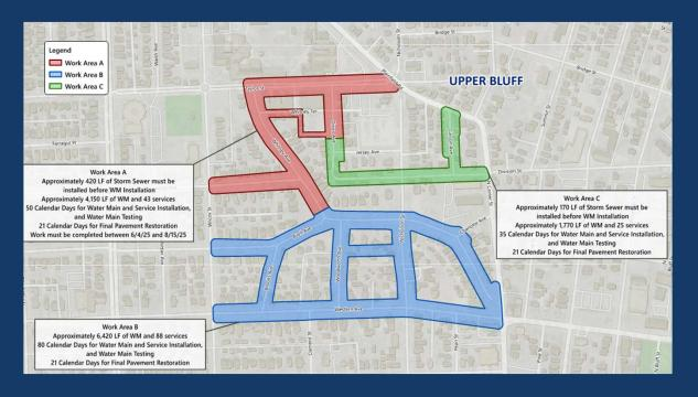
12,300 feet of 6" – 12", DI or PVC - Includes 1,000 feet of 8" via HDD
