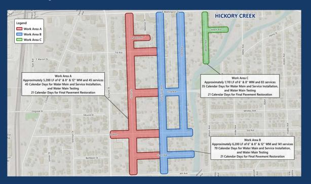
12,800 feet of 6" – 12", DI or PVC - Includes 800 feet of 8" via HDD
