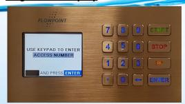
1. Using the Keypad, type in the Access code and then ENTER.
