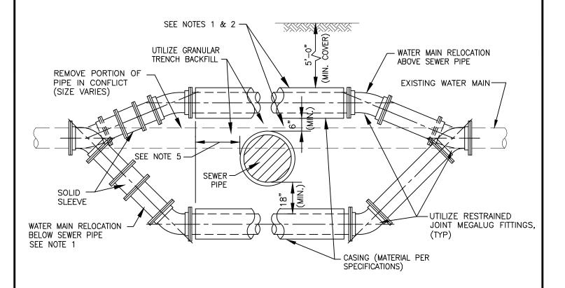
NOTES: 1. ONLY TO BE USED IF WATER MAIN CANNOT CROSS ABOVE PROPOSED SEWER AND MAINTAIN THE REQUIRED 18" OF SEPARATION AS SHOWN ON DRAWING, OR APPROVED BY ENGINEER IN FIELD.
