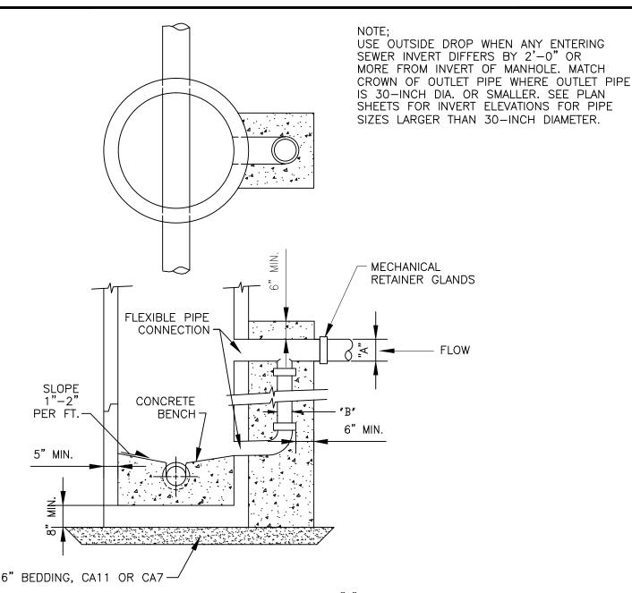
1. 8-INCH TO 12-INCH DIAMETER DROP: DUCTILE IRON CLASS 50. UTILIZE DUCTILE IRON RESTRAINED JOINT PIPE AND FITTINGS FOR DROP ELBOW, PIPE, AND TEE AT INCOMING SEWER. ENCASE ENTIRE DROP PIPE FROM BASE OF MANHOLE TO 6 INCHES ABOVE TOP OF INCOMING SEWER WITH 4000 PSI CONCRETE AT A MINIMUM THICKNESS OF 6 INCHES.
