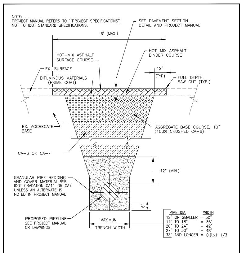
FOR PAVEMENT WITH AGGREGATE BASE AND COMPACTED GRANULAR BACKFILL MATERIAL
