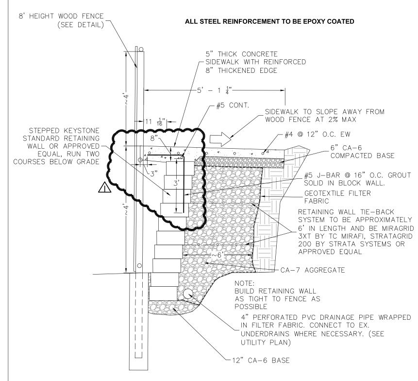
1. CONTRACTOR TO INSTALL PER MANUFACTURER'S RECOMMENDATIONS. 2. CONTRACTOR TO HAVE STRUCTURAL ENGINEER PROVIDE FINAL DESIGN FOR RETAINING WALL AND TIE BACK SYSTEM. PROVIDE SIGNED AND SEALED SHOP DRAWINGS BY IL SE. BID TO INCLUDE STRUCTURAL DESIGN REQUIREMENTS AND INCLUDE MORE STRINGENT DESIGN STANDARD THAN ABOVE AS NECESSARY
